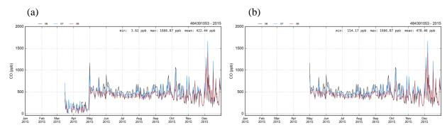
Figure 4. Preliminary time series analysis of Fort Worth near road site CO measurement data (a) with invalid data (before May 1, 2015) and (b) after the invalid data were removed.
