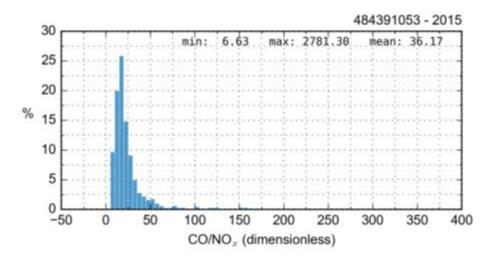
Figure 6. Preliminary ambient CO/NO<sub>x</sub> ratios for the Fort Worth near-road site.
